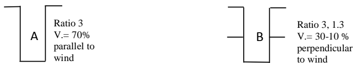
Fig.5. Section at streets with ratios and value of air velocity : (A) street that is parallel to wind direction; (B) street is perpendicular to wind (free air velocity 7m/s).
